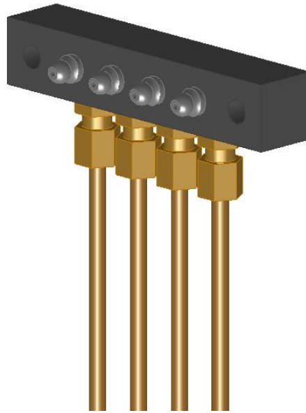
Fig. 10 Stage Header Block with Grease Lines Connected to it.
